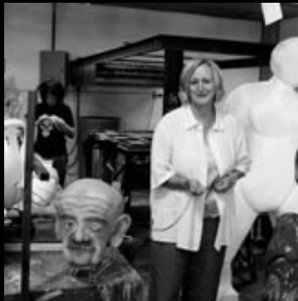
Zuanda Badenhorst, Chair of the Department of Entertainment Technology, Tshwane University of Technology, with an animatronic head developed in the E.T. Properties area. The eyes open and close, the mouth opens and shuts, the forehead wrinkles, the chin sinks, and the ears wiggle.
