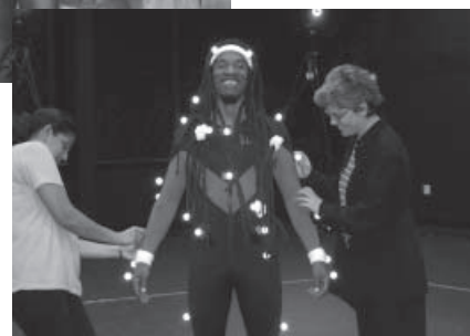
At the new ACCAD MoCap lab, Suba Varadarajan (left) and Maria Palazzi (right) help Benjamin into the motion capture suit. Each reflective marker represents a point that the computer will track.
